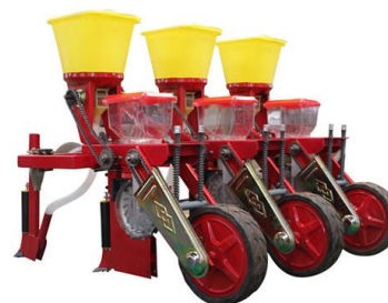
Fig 2: Tractor drawn maize planter
