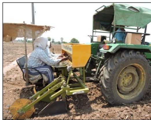
Figure 3: Raised bed turmeric semi-automatic planter
