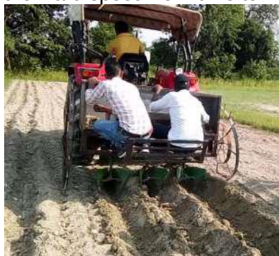
Figure 2: Semi-automatic turmeric planter
